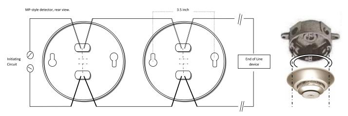
The detector is installed using rain-tight conduit and a standard, approved weatherproof electrical enclosure as shown above. A neoprene (or similar gasket supplied with the back box), is installed between the detector's seal plate and the back box. The wire leads are connected to the initiating circuit inside the enclosure. Unused threaded openings are sealed with threaded plugs. A decorative anodized aluminum cover ring snaps over the detector to complete the installation.
