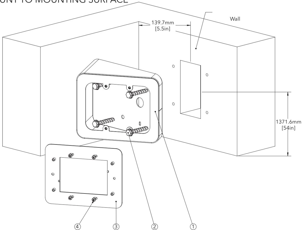
1. Use item No.1 to mark and drill installation holes to mounting substrate.
