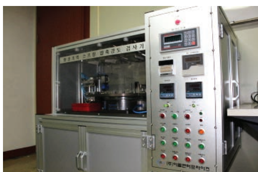
SMA Spring Inspection M/C
