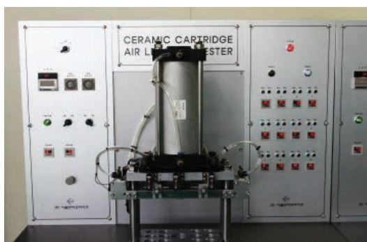
Air Leakage Inspection M/C
