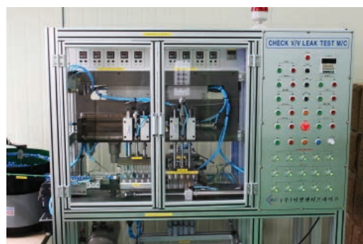
Check Valve Leakage Inspection M/C
