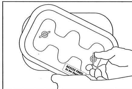
Loosen the knobs / wing-nuts, but do not remove the knobs / wing-nuts.
