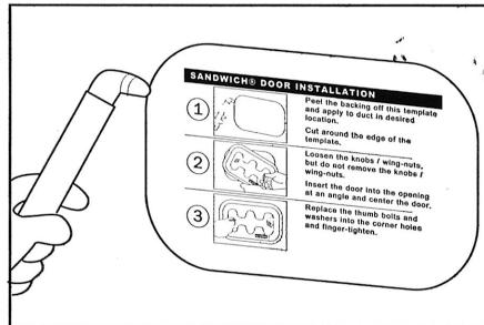
Peel the backing off this template and apply to duct in desired location.
