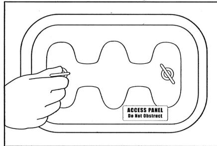
Finger-tighten the knobs / wing-nuts. Do not over-tighten.
