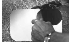
3. Insert door into opening at an angle and tighten knobs.
