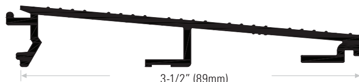
DS1135A150 Extruded aluminum mill finish. Length available: 150" (3810mm) only
