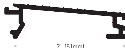
DS1128A150 Extruded aluminum mill finish. Length available: 150" (3810mm) only
