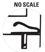
Required kerf slot size 5/64" (2mm) wide x 9/32" (7mm) deep
