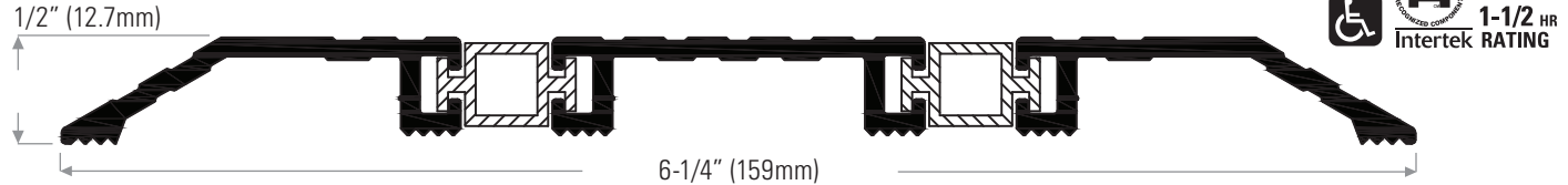
DS603TBA Extruded aluminum mill finish with 2 thermal breaks
