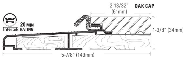
**DS578AOAK** Extruded aluminum sill mill finish with interior oak cap. Length available: 150" (3810mm) only
