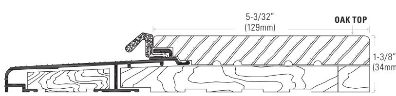
**DS858AOAK** Extruded aluminum sill mill finish, with interior oak cap. Length available: 150" (3810mm) only
