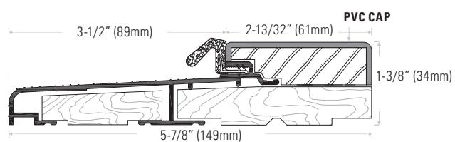
**DS578AVT** Extruded aluminum sill, mill finish with interior vinyl cap, tan. Length available: 150" (3810mm) only
