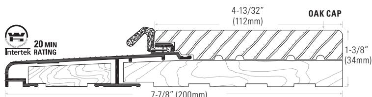
**DS778AOAK** Extruded aluminum sill, mill finish with interior oak cap. Length available: 150" (3810mm) only
