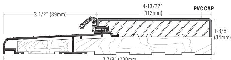
**DS778AVT** Extruded aluminum sill, mill finish with interior vinyl cap, tan. Length available: 150" (3810mm) only
