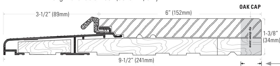
This section may be ripped down to any measurement between 8-3/4" (222mm) & 9-1/2" (241mm) to achieve a custom sill width
