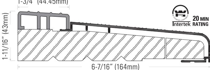
**DS612AHVT** Extruded aluminum sill, mill finish with fixed high vinyl cap, tan
