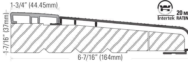
**DS612AVT** Extruded aluminum sill, mill finish with fixed vinyl cap, tan.
