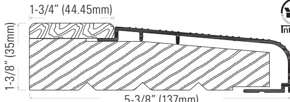
**DS512AOAK** Extruded aluminum sill mill finish with fixed oak cap
