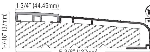
**DS512AVT** Extruded aluminum sill, mill finish with fixed vinyl cap, tan.
