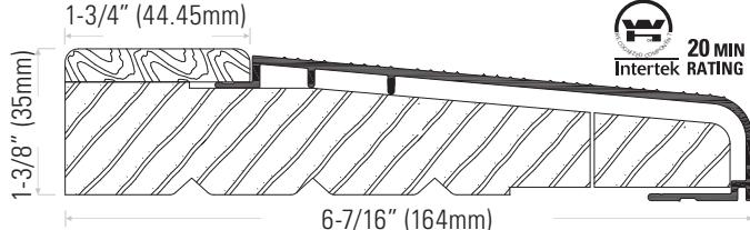
**DS612AOAK** Extruded aluminum sill, mill finish with fixed oak cap
