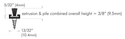
DS369A7535G Aluminum extrusion mill finish with fin pile insert, grey
