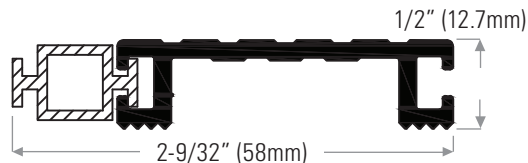
DS202TBA Extruded aluminum mill finish with thermal break insert
