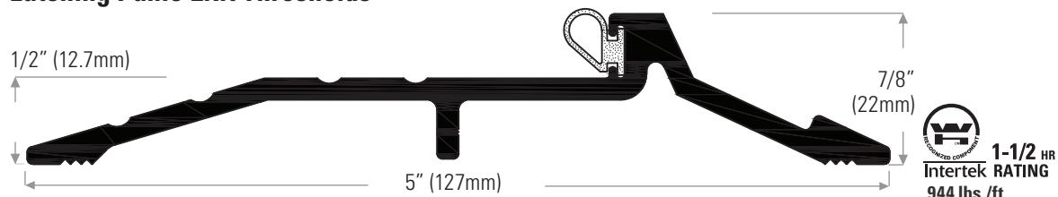
**DS177A** Extruded aluminum mill finish, no insert (rated)
