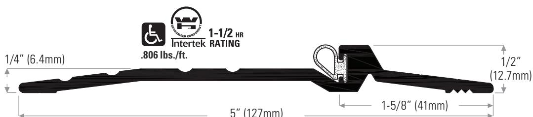
**DS178A** Extruded aluminum mill finish, no insert (rated)
