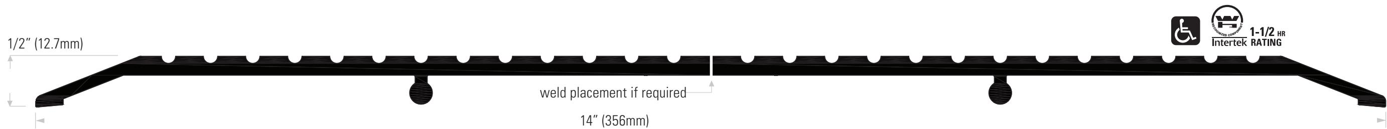
**DS1400HA** (2 piece) extruded aluminum mill finish, not welded
