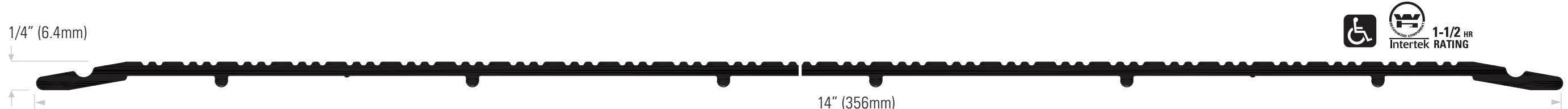
**DS14000A** (2 piece) extruded aluminum mill finish, not welded
