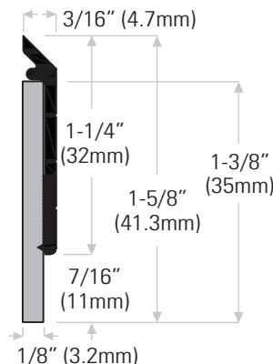
**DS138CN** Extruded aluminum clear anodized with rubber insert, black, 1/8" x 1-3/8" (3.2mm x 35mm)
