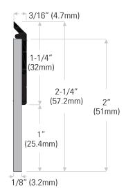
**DS138CN-2** Extruded aluminum clear anodized with rubber insert, black, 1/8" x 2" (3.2mm x 51mm)
