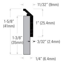
DS135CN Extruded aluminum clear anodized with 1/4" x 1-3/8" (6.4mm x 35mm) rubber insert, black
