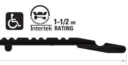
**DS12000A** (2 piece) extruded aluminum mill finish, not welded
