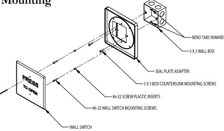
**Step 4:** Thread the enclosed #6-32 screws into the seal plate adapter, tightening until approximately 1/4" of the threads remain visible.
