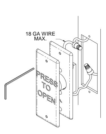
TIGHTEN SCREWS THROUGH HOLES IN COVER PLATE WITH HEX KEY PROVIDED
