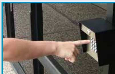
Digital Keypad Code Entry Enter 4 or 5-digit unique PIN to gain entry, up to 1000 4-digit entry codes
