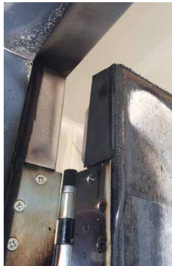
The intumescent kicked in, sealing the door and smoke successfully.
