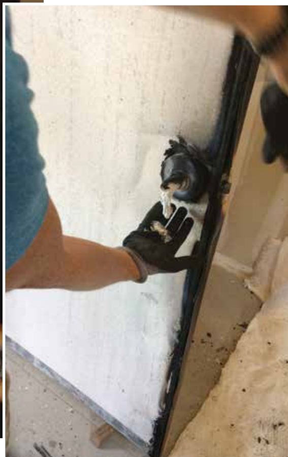
Close up of what a cylindrical lock handle looks like after 15 minutes of 2,000 F. Still latched.
