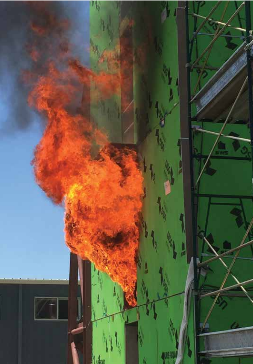
Second floor corridor burn. The fire was set on the other end of the building, but most of the flames traveled down the corridor out this other side.
