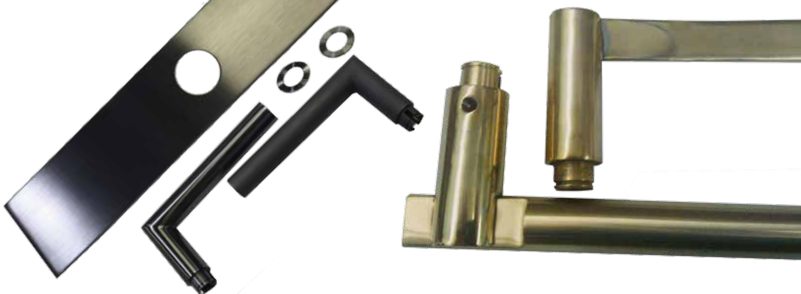
PVD black on satin, matte, and polished stainless steel surfaces. PVD process does not change surface texture, so these were all run in the same chamber.
