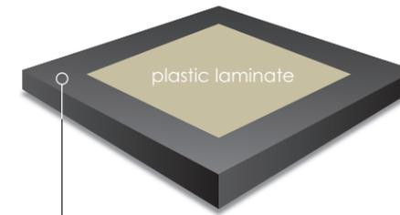
The 50 mm (2") solid phenolic edges prevent moisture penetration and ensure greater strength to install hardware and accessories.
