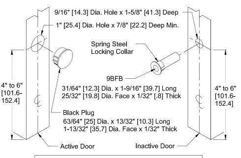
IMPORTANT: The 9BFB will project during a fire. Do not cover with any edge mounted door hardware.
