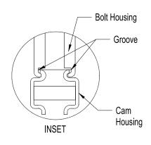
If Cam Housing rotates, it is not engaged into the Bolt Housing.
