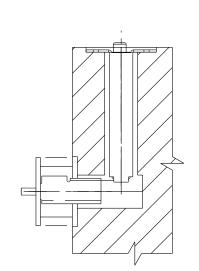
3. Adjust Bolt Head 0" to 1/2" [12.7] above Bolt Head Guide. Secure with 2 ea. #8 APS
