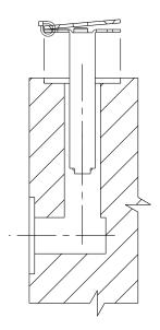
2. Install Cam Housing into grooves of Bolt Housing. See Inset. Secure Trim Plate with 2 ea. #8 APS
