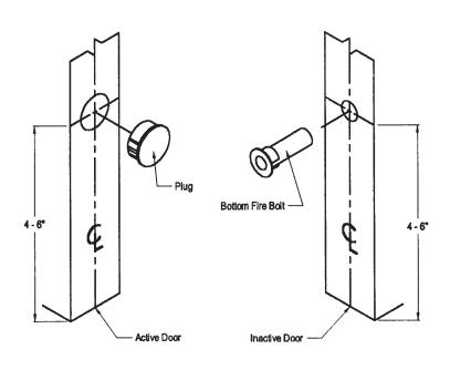
The 805, 840, 905, 940, and 960 Automatic and Self Latching Top Flush Bolts are UL Listed for pairs of fire doors when specified with the 8BFB or 9BFB Bottom Fire Bolt.
