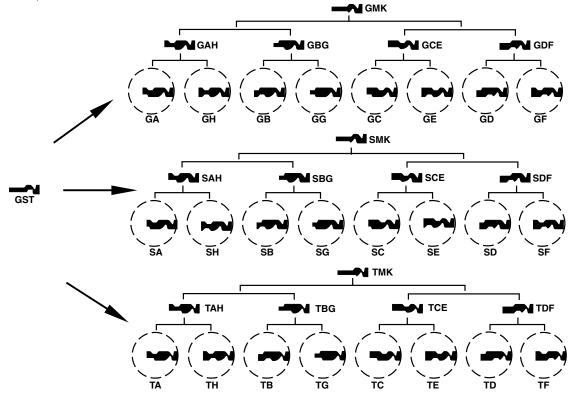
Note: The section of the key is determined by viewing the key from the bow towards the tip.
