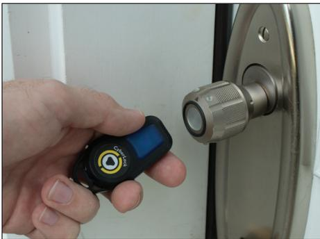
Open FlashLock using an infrared key fob.
