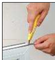
Cut to length with knife or scissors
