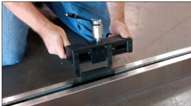
Fully Insert the TAPER-LOC™ Tapers and Lock Them into Place with the TLK5 Installation/Removal Tool
