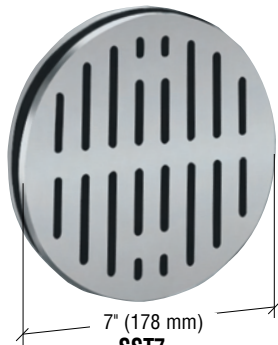
SST7 Requires 4-1/2" to 6" (114 to 152 mm) Hole. Uses Four Screws (Included)
