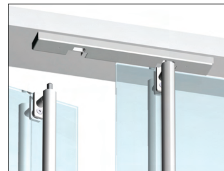
Glass Mount Detail at Latch With Header and ESK Strike
