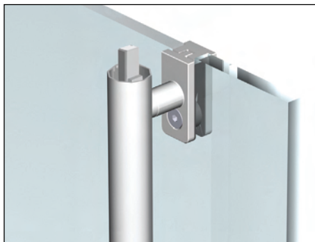
Glass Mount Detail at Latch
