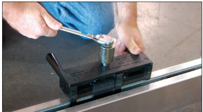
Fully Insert the TAPER-LOC™ Tapers and Lock Them into Place with the TLK5 Installation/Removal Tool
