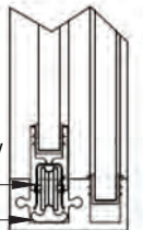
Ball Bearing Wheel Assembly
