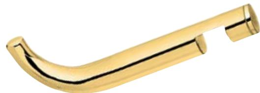
The solid brass Designer Series Sleeve-Over Robe Hook mounts on the top of 1/2", 3/8" or 5/16" (12, 10, or 8 mm) glass without the need for drilling or notching the glass. It can be positioned anywhere you want along the top of the glass, and is secured in place by tightening a nylon-tipped Allen set screw. Clear gaskets are included.
