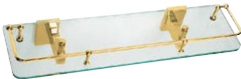
Beautiful 5/16" (8 mm) thick glass shelf has polished flat edge with arrises, and measures 18" x 5" (457 x 127 mm). Supported by two Geneva style wall-mounted brackets with concealed fasteners.
