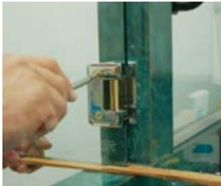
Loosen the cover plate and align the door.
