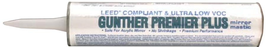
Gunther Premier® Plus at 72°F (22°C) achieves approximately 30 percent strength in 24 hours, full cure in 7 days. Gunther Premier® Plus should be applied in 3/8" (9.5 mm) vertical beads, 5 to 6" (127 to 152 mm) apart and away from the edge to prevent squeeze out. Approximate coverage is 7 sq. ft. per cartridge.
