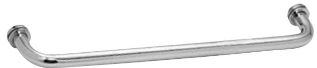
These Single-Sided Towel Bars are designed for use on frameless glass doors or fixed panels. Bars are made from 3/4" (19 mm) diameter brass tubing, and come with matching finish metal washers. The narrow inside End Caps protrude only 1/4" (6 mm) from the glass surface.
