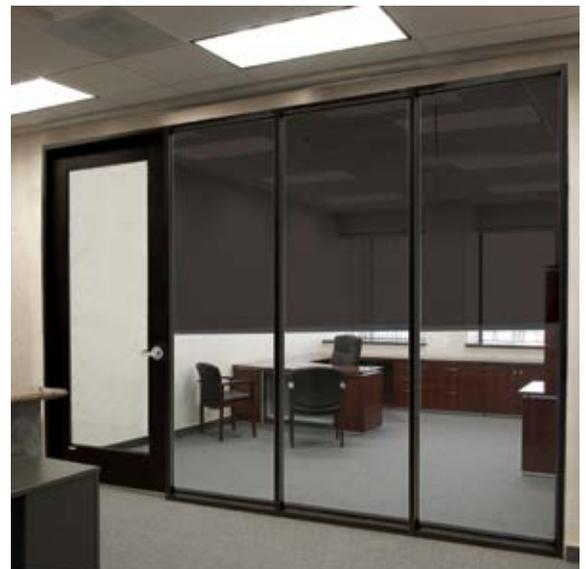
The 487 Series 3" (76 mm) Offset Glazed System offers the same advantages as our 1-1/2" (38 mm) Trim Series with a 1-1/2" x 5-11/16" (38 x 144 mm) frame that accepts a variety of glass thickness in an offset position, allowing for recessed window coverings and blinds.
