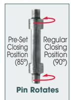
Hinges come with the 90° side activated. Pre-Set Models come with the Pin pre-set for 85° (5° tighter closure into shower interior). The Pin can be rotated (not flipped upside down) to activate the other side.
