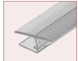
'Y' Inline Panel Seal is for use on 180° inline glass-to-glass applications. Snap onto the fixed panel with the lip on the strike side. Soft vinyl helps cushion door closure.
