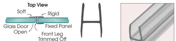
Versatile Multi-Purpose 'H' Wipe has two rigid legs and two soft legs. It can be used as a bottom sweep, or as a seal if run vertically up the edge of the door. One or both soft legs can be trimmed to accommodate many installation options.
