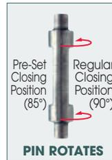
Each Trianon Hinge contains a Reversible Pivot Pin. One side of the Pin is marked at 90°. The opposite side of the Pin is marked 85°, which allows 5° tighter closure into shower area. The Pin can be rotated (not flipped upside down) to activate the other side.
