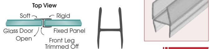
Our NEW Multi-Purpose 'H' Wipe With "Extra Soft" Twin Legs acts as a versatile seal that can be used either on the side or bottom of a door. Because of the very soft dual legs, quieter door closure can be expected, as opposed to closing into harder plastic seals. It is also easy to trim the very soft legs to accommodate your particular application.
