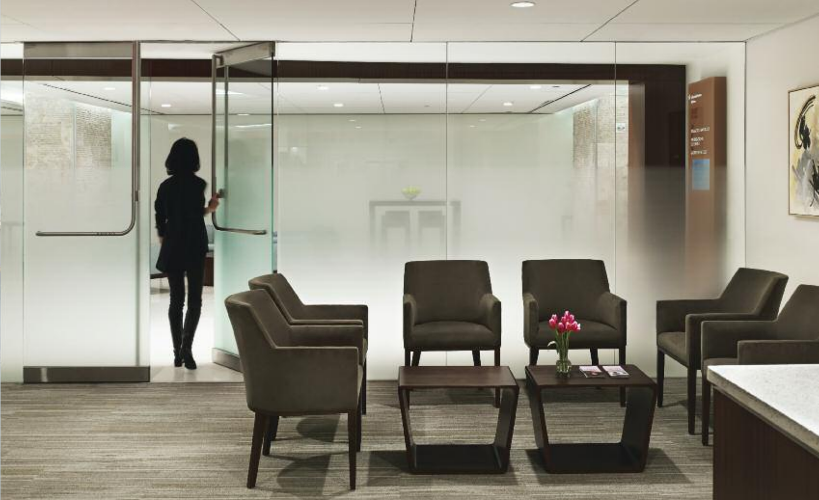
CRL Clear View Pivoting System in Brushed Stainless with CRL-Blumcraft® PA100-F Series Panic Handles.
