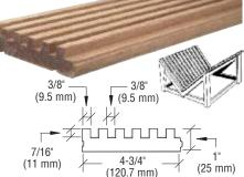
The finest grade of clear grain hardwood is accurately milled and used for this flooring as it provides long wear and easy glass handling. You can make your own harp rack with Slot Rack Flooring or use it to make a "V" shaped rack for cut off pieces. Simply lay lengths on the floor – they are grooved to join together snugly without nails or other fasteners. Minimum order is one 12' (3.66 m) length. Must ship common carrier. **NOTE**: Not Available in Australia.
