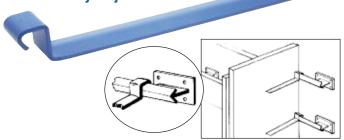
CRL Glass Case Brackets are an economical and simple way to keep cases of glass organized. Just mount a stand-off 1-1/2" x 1-1/2" (38 x 38 mm) angle-iron on a blank wall and hang the Case Bracket wherever you need them to hold cases upright. They are made of steel, and are 18" (457 mm) long. We suggest cases be supported near the top and bottom. Minimum order is one each.
