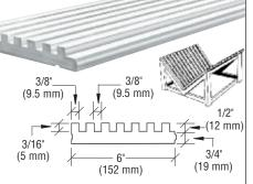
CRL High Density PVC Slot Rack Flooring is precision milled with 3/8" (9.5 mm) wide by 3/16" (5 mm) deep grooves to provide quality replacement rack flooring or to provide a base for racking of your own design. This 1/2" (12.7 mm) PVC material, bonded onto 3/4" (19 mm) OSB board, provides the ultimate in low friction slide storage systems. Minimum order is one 96" (2.44 m) length. Must ship common carrier.
