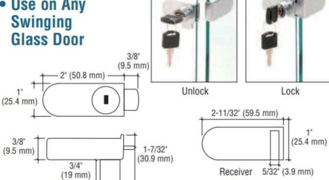
This CRL No-Drill Showcase Lock is designed for swinging glass doors, and is easily installed by peeling off the adhesive liner and placing the Lock and Receiver in the desired location on the glass. No drilling or notching of glass is required. The No-Drill Lock can be used on any thickness of glass door or showcase. Available in several different finishes to match popular showcase extrusions. Can be ordered keyed randomly or alike.
