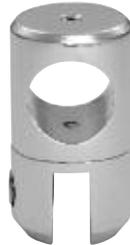
The Adjustable Support Bar Bracket is for use with only 1/4" or 5/16" (6 or 8 mm) thick tempered glass thicknesses. It is installed at the top of the glass and swivels to accommodate various angles. Simply secure to the end of a S1, S2 or S80 length Support Bar.
