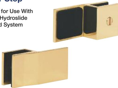
The Door Stop for CRL's Hydroslide Bifold Hinge System will protect the shower door from closing too far and damaging the door. The solid brass constructed Door Stop is dimensioned to accept 3/8" and 5/16" (10 and 8 mm) thick tempered glass when used in conjunction with our Hydroslide Bifold Hinges (HYDH037 and HYDH180). No glass fabrication is required.
