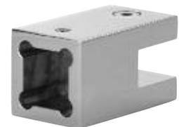
This Square Cornered Support Bar Bracket mounts on top of a fixed panel of glass with the attached support bar extending in an upward direction to the ceiling. Use with Cat. No.'s SQ39 or SQ59 Bars. Wall mounting bracket is ordered separately for mounting to the ceiling.
