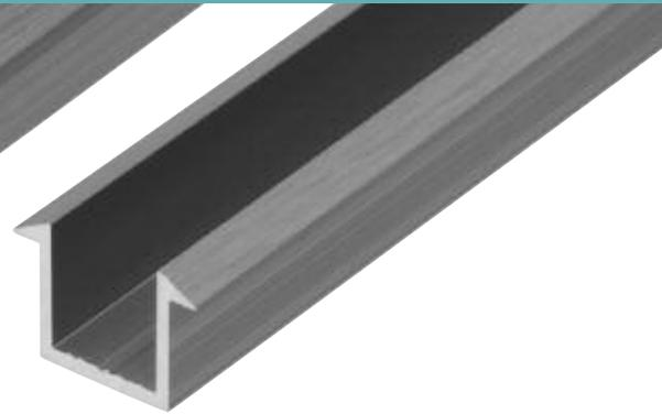
This U-Channel is the ideal selection for recessing into the floor, wall, or ceiling to provide the frameless "all-glass" appearance. The top lip of the U-Channel is angled to deflect the water away and conceal the edge of the tile. Glass is wet glazed into the Channel. 98" (2.49 m) stock lengths are available for 3/8" or 1/2" (10 or 12 mm) tempered glass.
