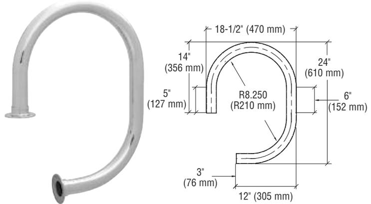
CRL Counter Mount Service Rails are easily secured with screws and CRL Cat. No. 32629 Metal Contact Cement (see page P602). The Rails can be field cut for fitting to your particular installation needs. Each Rail is supplied with six #10 x 1-1/2" (38.1 mm) Flat Head Wood Screws.
