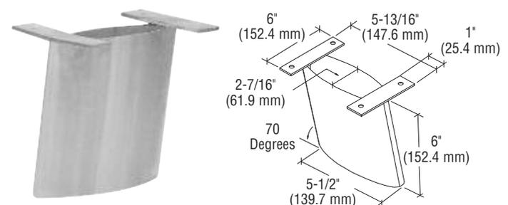
CRL's Angled Supports have the same height and width dimensions as the Vertical Support, but project at a 2" (51 mm) angle from bottom to top for installation of cantilevered stone bar tops. These elegantly styled Supports will provide the finishing touch for custom granite counters. Minimum order is one each.
