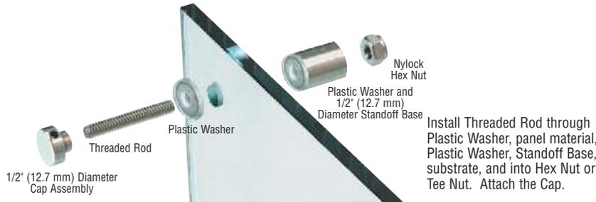
Install Threaded Rod through Plastic Washer, panel material, Plastic Washer, Standoff Base, substrate, and into Hex Nut or Tee Nut. Attach the Cap.
