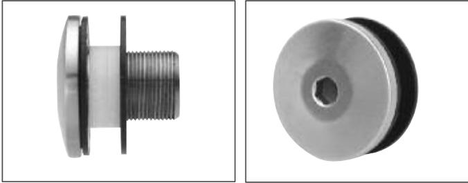
CRL Surface Mount Cap Assemblies work with eight different Column or Arch Swivel Fittings. Each Cap is supplied with all necessary gaskets. Fittings are tightened with a 6 mm Allen wrench (not supplied). Thread pitch is M18 x 1 mm. See below for glass fabrication requirements.
