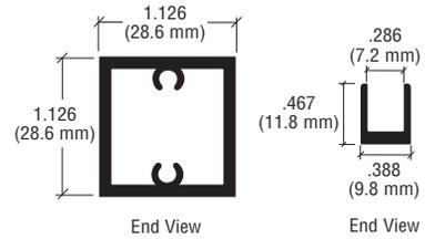
These fully assembled Design Series Posts measure 1-1/8" (28.6 mm) square. Post Mounting Base Plates measure 2" (50.8 mm) square. Glazing Channels measure full length and rise 15/32" (11.8 mm) from the post surface. Glazing Vinyl for 1/4" (6 mm) and 3/16" (5 mm) glass is supplied to fill glass channel.
