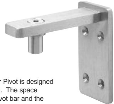
This CRL Wall Mount Door Pivot is designed for mounting to a post or wall. The space between the bottom of the pivot bar and the CRL Top Door Patch Fitting (not included) has been reduced to 1/8" (3 mm), because at gate height the chance of pinching fingers is greatly reduced. Available in brushed stainless steel finish, complete with instructions and a glass cut-out template. Minimum order is one each.
