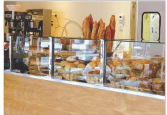
CRL 1-1/2" Square Plaza Series Sneeze Guards are available in 12", 18", and 24" (305, 457, and 610 mm) heights with a 12" (305 mm) Top Shelf. Five styles are offered, Right Hand Open End, Left Hand Open End, Center Open, Left Hand Closed End, and Right Hand Closed End. Standard finishes are brushed stainless and polished stainless.
