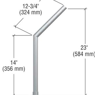
Our Open Front, Glass On Slant Elegant Series Sneeze Guards are in stock and ready for immediate shipment. The 2" (50.8 mm) Tubing is available in three styles that easily attach to the counter. Ships fully assembled.
