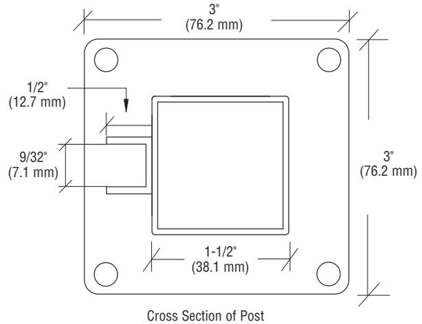
Posts measure 1-1/2" (38.1 mm) square; Welded base plates measure 3" (76.2 mm) square; 1/4" (6 mm) glazing channels measure full length, and rise 1/2" (12.7 mm) from the post surface.
