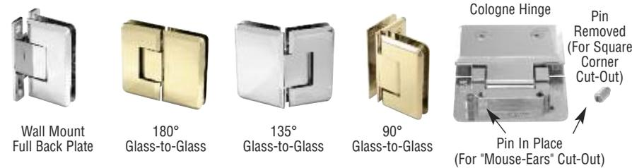
Vienna and Cologne Series Hinges are ideal for wider and heavier doors. Two hinges can accommodate up to a 36" (914 mm) wide door weighing up to 110 pounds (49.9 kg), while three hinges can accommodate up to a 36" (914 mm) wide door up to 140 pounds (63.5 kg).
