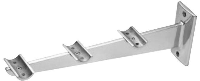
CRL Tray Slide Shelf Brackets have a 12" (305 mm) projection and support three evenly spaced 1" (25.4 mm) tubes. Maximum Shelf Bracket spacing is 42" (1067 mm) apart. Additional information available at [crlaurence.com](http://crlaurence.com).
