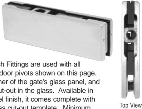
CRL Top Gate Patch Fittings are used with all three of the gate and door pivots shown on this page. It fits in the upper corner of the gate's glass panel, and requires a hole and cut-out in the glass. Available in brushed stainless steel finish, it comes complete with instructions and a glass cut-out template. Minimum order is one each.
