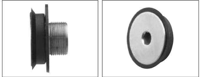
CRL Flush Mount Cap Assemblies work with eight different Column or Arch Swivel Fittings. Each Cap is supplied with all necessary gaskets. Fittings are tightened with a 6 mm Allen wrench (not supplied). Thread pitch is M18 x 1 mm. See below for glass fabrication requirements.
