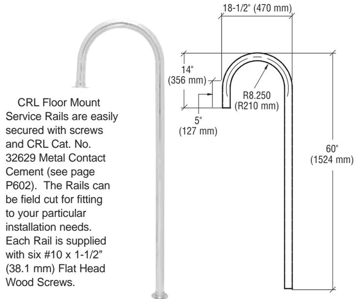
CRL Floor Mount Service Rails are easily secured with screws and CRL Cat. No. 32629 Metal Contact Cement (see page P602). The Rails can be field cut for fitting to your particular installation needs. Each Rail is supplied with six #10 x 1-1/2" (38.1 mm) Flat Head Wood Screws.
