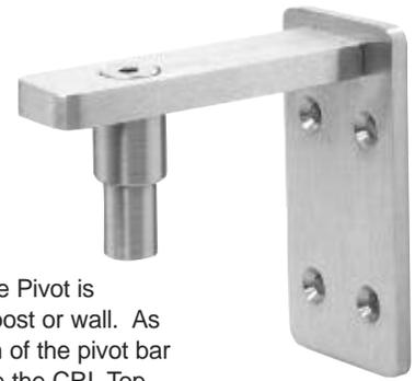
This CRL Wall Mount Gate Pivot is designed for mounting to a post or wall. As a safety measure the bottom of the pivot bar is raised 3/4" (19 mm) above the CRL Top Gate Patch Fitting (not included), allowing for adequate space to help prevent pinching of fingers. Available in brushed stainless steel finish, it comes complete with instructions and a glass cut-out template. Minimum order is one each.
