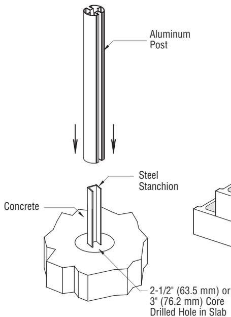
**Core Mounted Installation for CMU Block Walls**
