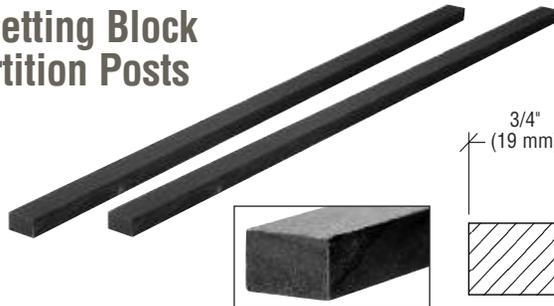
This Post Setting Block fits into the glass pocket to support the glass panel at the height you determine. It is made of a rigid UHMW plastic composite that won't compress under the weight of the glass, helping to maintain an even sight line. You can trim it to any length you require.
