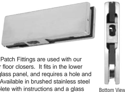
CRL Bottom Gate Patch Fittings are used with our bottom door pivots or floor closers. It fits in the lower corner of the gate's glass panel, and requires a hole and cut-out in the glass. Available in brushed stainless steel finish, it comes complete with instructions and a glass cut-out template. Minimum order is one each.
