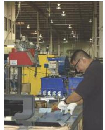
**Fixtures and Welding** - Precise and accurate fixtures guarantee constant and repetitive results. Having all component parts securely fastened prevents warping and mis-alignment during the welding process.
