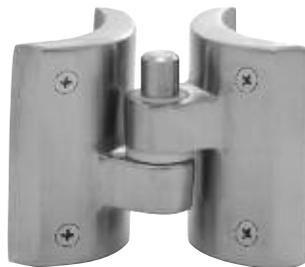
This CRL Tubing Hinge is designed to work with 1.9" (48.3 mm) diameter tubing. The Hinge is free-swinging, and pivots on a nylon bearing. Hinge is secured from the front side with supplied screws. Maximum width 42" (1067 mm); maximum weight 65 lbs. (29.5 kg). Minimum order is one each.
