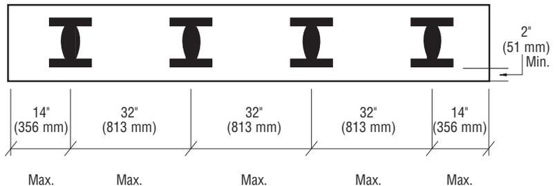
Measure top of bar to determine the number of Supports required. Maximum recommended distance from ends is 14" (356 mm) on center. Distance between center Supports should be no greater than 32" (813 mm) on center. Minimum distance from the edge of the bar top is 2" (51 mm), as shown above.
