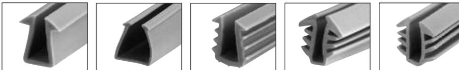
CRL Glazing Vinyls are made to fit D631 Glass Channel, normally used for 1/4" glass, to accommodate glass or other glazing materials 7/32", 3/16", 1/8" or 1/16" thick. When glazing is completed, all that remains visible is a neat "bead" that gives the framed glass or other glazing material a finished professional appearance. Available in gray color only.
