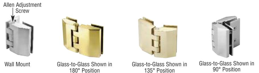
The Regal Hinge offers an adjustable closing angle from 0 to 90 degrees. After the door is installed, simply loosen the Allen screw adjustment, position the door to the desired closed position, and tighten the Allen screw.
