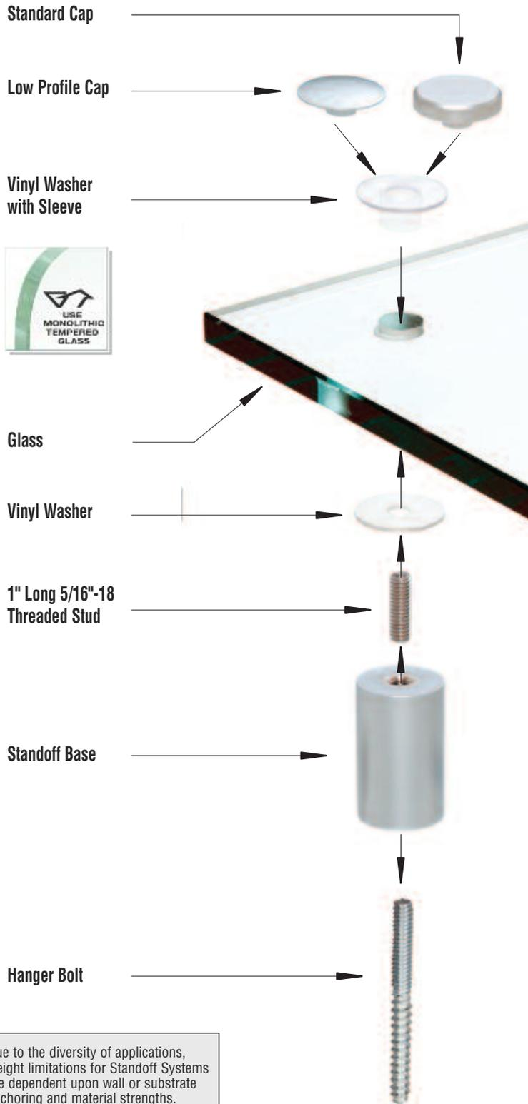
Due to the diversity of applications, weight limitations for Standoff Systems are dependent upon wall or substrate anchoring and material strengths.
