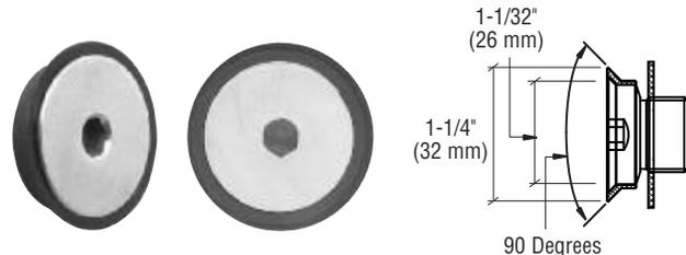
For CRL Flush Mount Caps use our Cat. No. PDT1 1" (26 mm) diameter Metal Bond Diamond Drill to make the required hole, and the Cat. No. BDC112 1-1/2" (38 mm) diameter Belgian Mount Diamond Countersink for the desired countersink depth stopping at 1-1/4" (32 mm) diameter. Thread pitch is M18 x 1 mm. Glass thickness range is 3/8" to 1/2" (10 to 12 mm).
