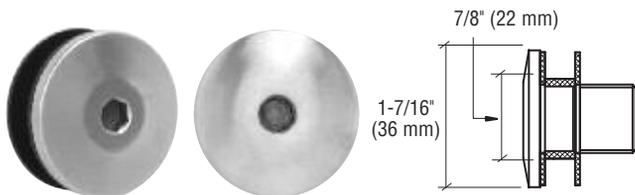
For CRL Surface Mount Caps use our Cat. No. PDT78 7/8" (22 mm) diameter Metal Bond Diamond Drill to make the required hole. Thread pitch is M18 x 1 mm. Glass thickness range is 3/8" to 1/2" (10 to 12 mm).
