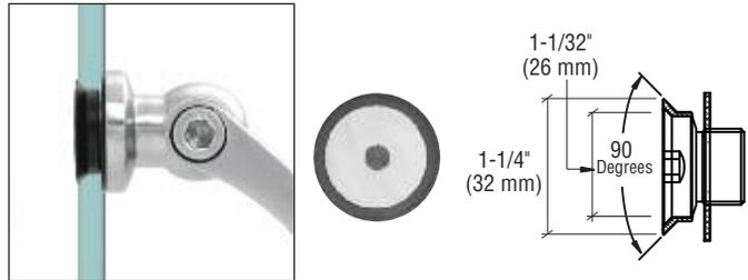
For CRL Flush Mount Caps use our Cat. No. PDT1 1" (26 mm) diameter Metal Bond Diamond Drill to make the required hole, and Cat. No. BDC112 1-1/2" (38 mm) diameter Belgian Mount Diamond Countersink for the desired countersink depth, stopping at 1-1/4" (32 mm) diameter. Glass thickness range is 3/8" to 1/2" (10 to 12 mm).
