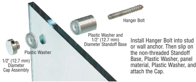
Install Hanger Bolt into stud or wall anchor. Then slip on the non-threaded Standoff Base, Plastic Washer, panel material, Plastic Washer, and attach the Cap.
