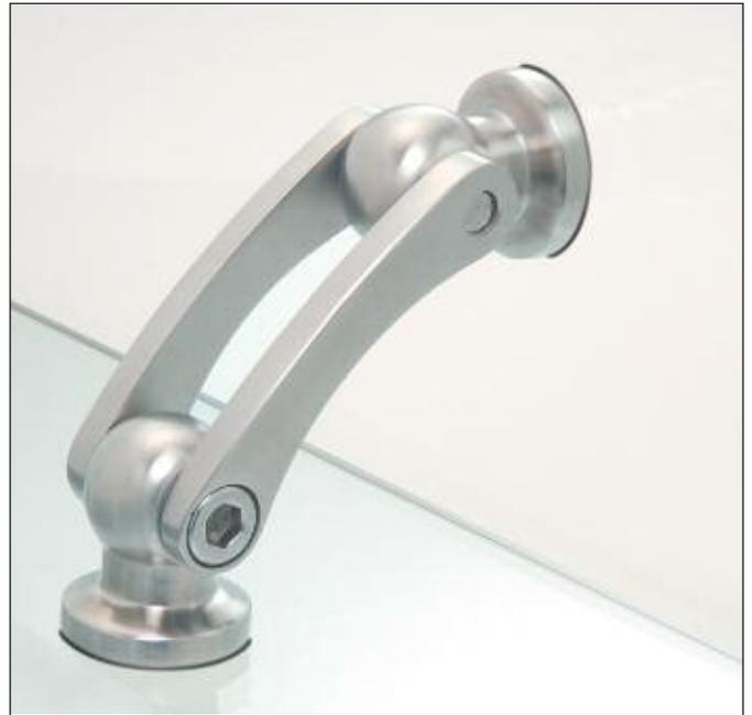
CRL's Arch Series Swivel Fittings are designed to provide a simple solution to connecting pieces of glass at different angles. Pivot angles for the Arch Series Swivels can be adjusted and locked into position by using a 5/16" Allen wrench (not supplied). The Arch Swivel Fitting gives you the option of selecting either a Surface Mount Glass Attachment Cap or a Flush Mount Glass Attachment Cap.
