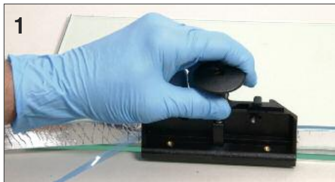
Apply Super Spacer® to clean glass surface with SSHN Hand Notcher or SSAPA Shuttle Applicator as release liner is removed.
