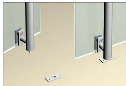
Glass Mount Detail at Bolt With 777SP Flat Strike
