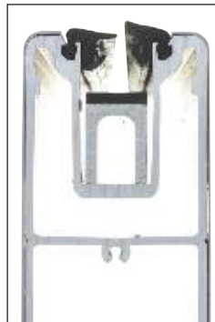
Top Load E.P.D.M. Glazing Gasket
