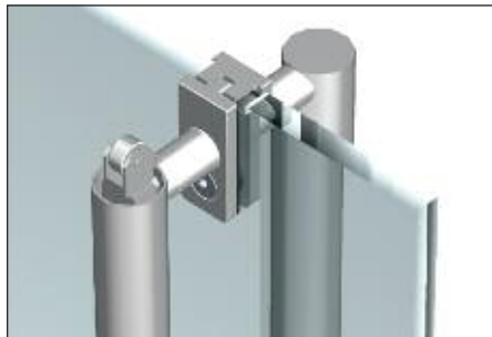
Glass Mount Detail at Latch
