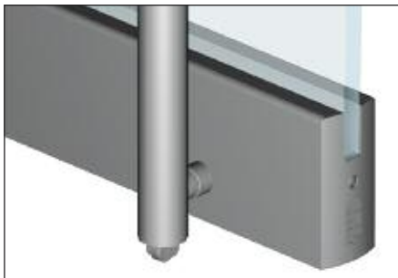
Rail Mount Detail at Latch
