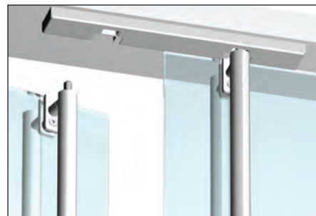
Glass Mount Detail at Bolt With Header and ESK Strike (Only for Optional Deadbolt Roller Catch)
