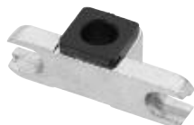
1NT303R Insert (Ordered Separately) for Rixson 340 Center Hung Walking Beam Pivot 1/2" (13 mm) Pin
