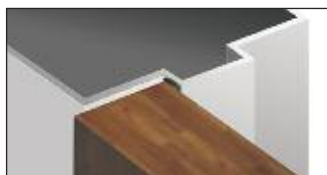
Compresses When Door is Closed
