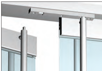
Rail Mount Detail at Bolt With Header and PK Strike
