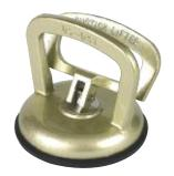
The split-handle design of the CRL Aluminum Single Pad Vacuum Lifter allows you to securely attach the pad to surfaces by simply pressing against the glass, then squeezing the two handle sections together. Also suitable for slightly curved or textured surfaces. The pad diameter is 4-1/2" (114 mm). Minimum order is one each.
