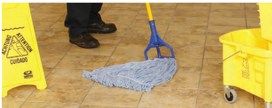
Use stirrup style mop handles with narrow band mops; Use jaws style mop handles with wide band mops.
