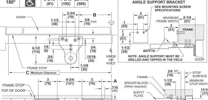
STOP WIDTH 11/16 (1) 3/8 754F25 (10)**Drop Plate** 3/8 5-1/8 (10)(130)(76)SEE MOUNTING SCREW **SPECIFICATIONS** 11-5/8 (295)**DOOR** (76)Drill thru 9/32 (7) Enlarge to 3/8 (10) Dia.-This Side Only (4 Places)
