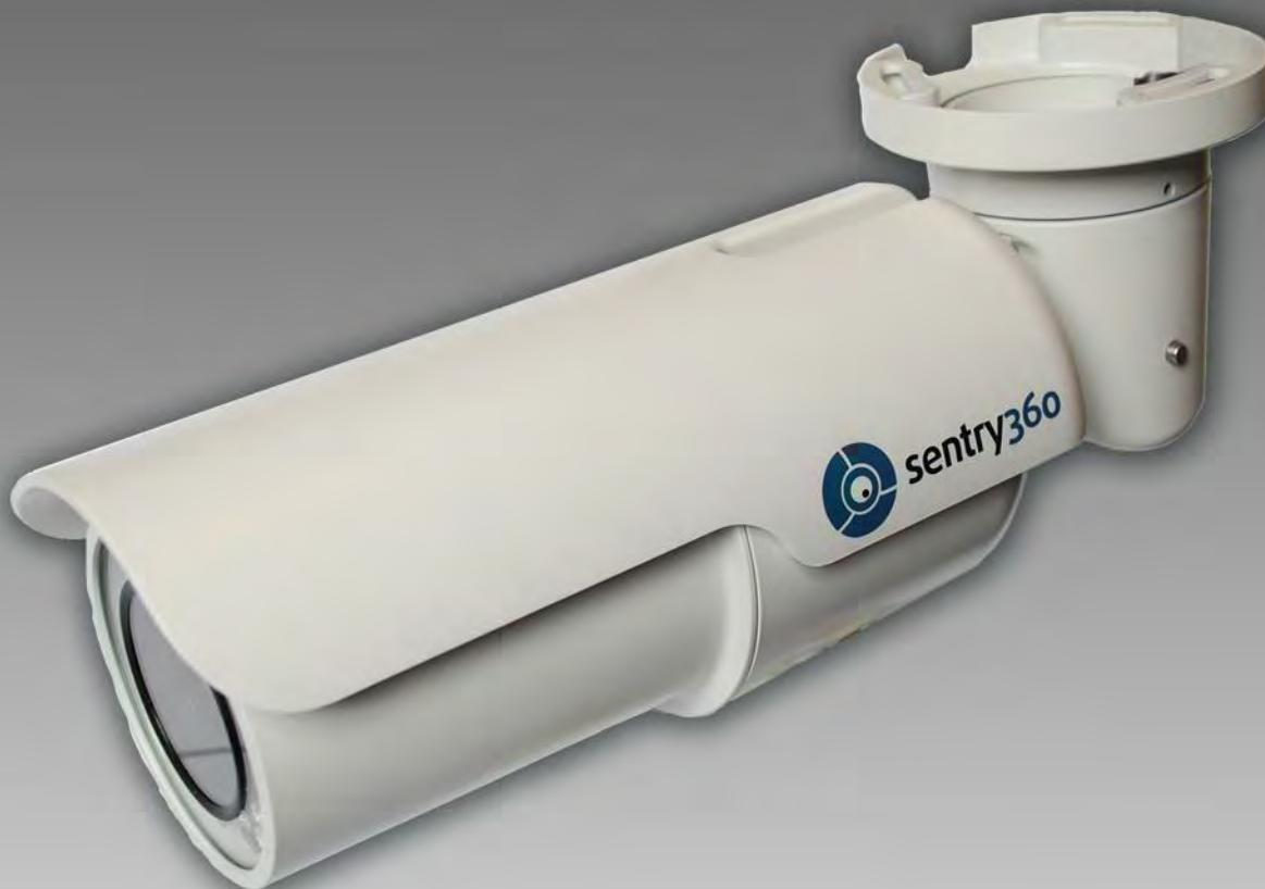
The IS-IP300-IRB camera is a Quad-streaming, H.264 & MJPEG encoding, 3.0 Megapixel resolution, IP-addressable, network camera. It is designed to deliver full-motion, high-definition, progressive scan digital video across local area networks. The IS-IP300-IRB features a design with no moving parts, a 1/2.7" CMOS sensor, Power over Ethernet, 23 built-in IR-LEDs, and Audio-In/Audio-Out. The IS-IP300-IRB is a cost effective, high-level, megapixel network camera.
