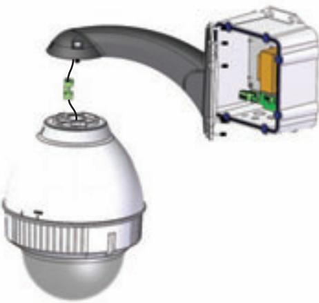
**Additional wires are provided to run power to PB24. Use with connector supplied. Run RJ45 connector through PB24, wall mount, and connect lead from housing.**
