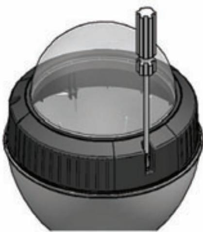
**Fasten down the dome with a Phillips screwdriver.**
