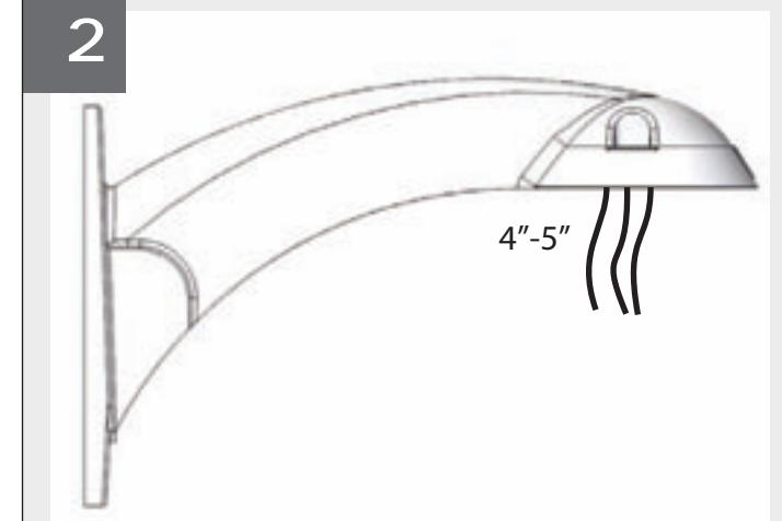
**Trim incoming control & power wires to 4" - 5", for either wall or pendent bracket**
