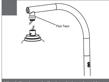
Attach the dome to the bracket, make wiring connections according to manufacturer.
