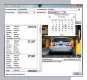
The VE410 provides out-of-the-box Automatic License Plate Recognition (ALPR) functionality using analog or network cameras. It can be used for various fixed parking applications, electronic toll collection or pay-per-use roads. License plates and their corresponding images are stored and can be easily searched. Various alarm scenarios can be achieved by using white or black lists.
