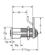
No.15783\* No. 15790\* **Distance Under Distance Under** Cam Cam Head to Cam Head to Cam No. Length B B<sup>1</sup> B⁰ B 1 5/16 205 1 3/16" 1 1 1/8" 206 25/32" 1 3/32" 207 1 1/8" 11/16" 1" 208 1 1/4" 9/16" 7/8" 209 1 7/16" 1" 1 5/16" 29/32" 210 15/16" 1 7/32"
