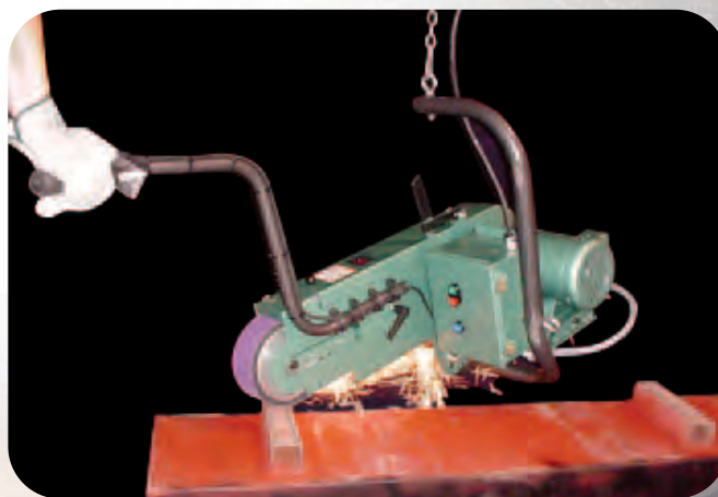
Model 979 adapts as a swing grinder.
