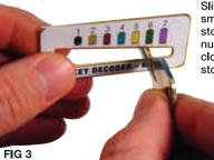
Slide the key towards the smaller end until the key stops and note the pin number directly above or closest to where the key
