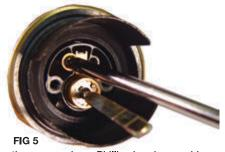
Remove the screw using a Phillips head screwdriver and
