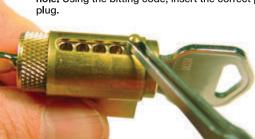
For example, if the bitting code is 43664 ...insert pin #4 into the first hole, pin #3 into the second hole, and pin #6 into the third hole, and likewise for the remaining chambers.
