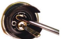
Replace the cylinder in the housing and insert the retaining screw. Check for proper function.
