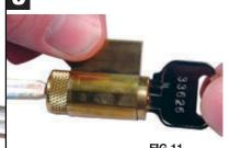
Dump the pins out. It may be helpful to move the key slightly back and forth to help eject the pins (FIG 11).
