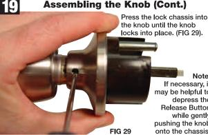
Note: If necessary, it may be helpful to depress the Release Button while gently pushing the knob onto the chassis.
