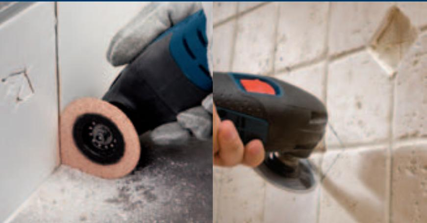
Applications for this Bosch lineup range from grout removal between closely set tiles to cutting abrasive materials. High-quality carbide grit and diamond-grit blades deliver great performance. Segment blades and a triangle rasp ensure Bosch grinding products can perform any application with precision in tight spaces.
